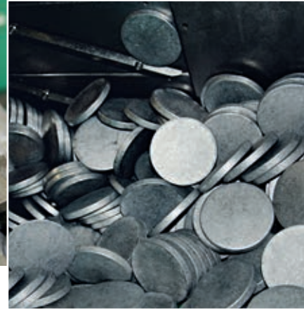
During the production process, each of these aluminium disks, so-called "slugs", becomes an aluminium bottle.
