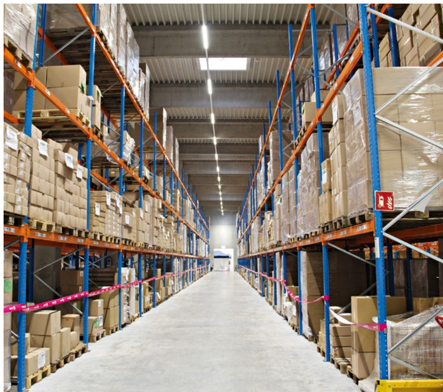
The new partially automated, high-bay warehouse offers around 5,500 pallet spaces.
