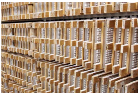
The shapes with the freshly cast fruit are brought to a specially air-conditioned hall to dry.
