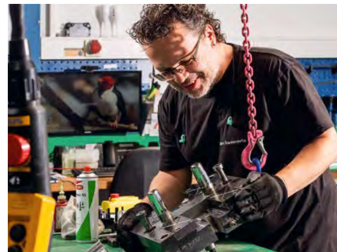
The injection moulds must be cleaned and maintained regularly. The moulds are dismantled into their individual parts for cleaning and repair.
