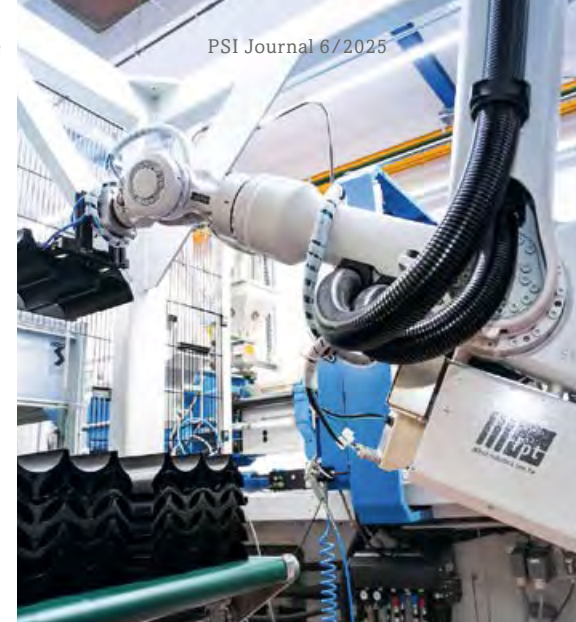
The handling device (robot technology) removes the finished moulded part from the machine and places it on a conveyor belt to cool down.
