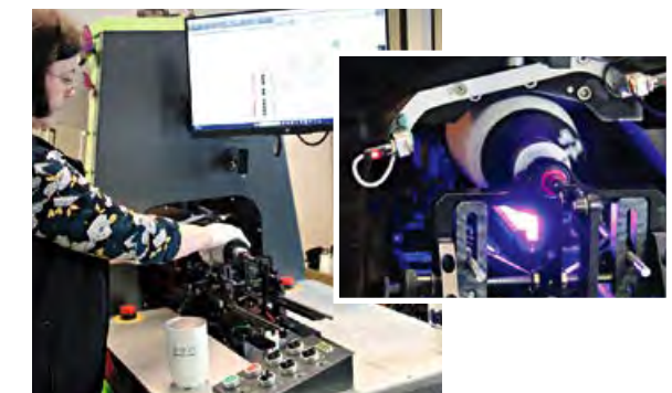
Here, cups are printed all the way around at 360°.
