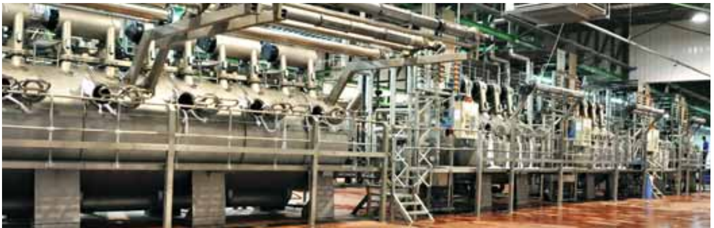
Fully automated: computer controlled dyeing plants.
