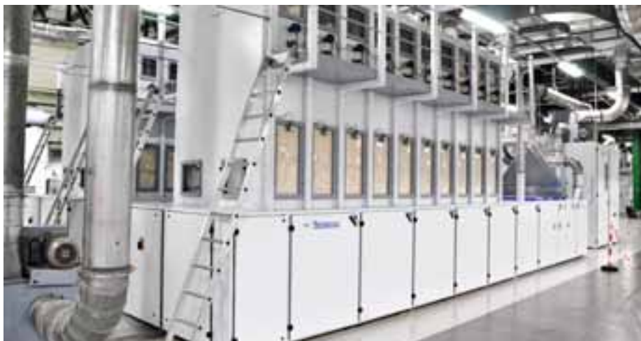
Fine mixture: The cotton bales are cleaned of all residual dirt and insects in the Blendomat production.
