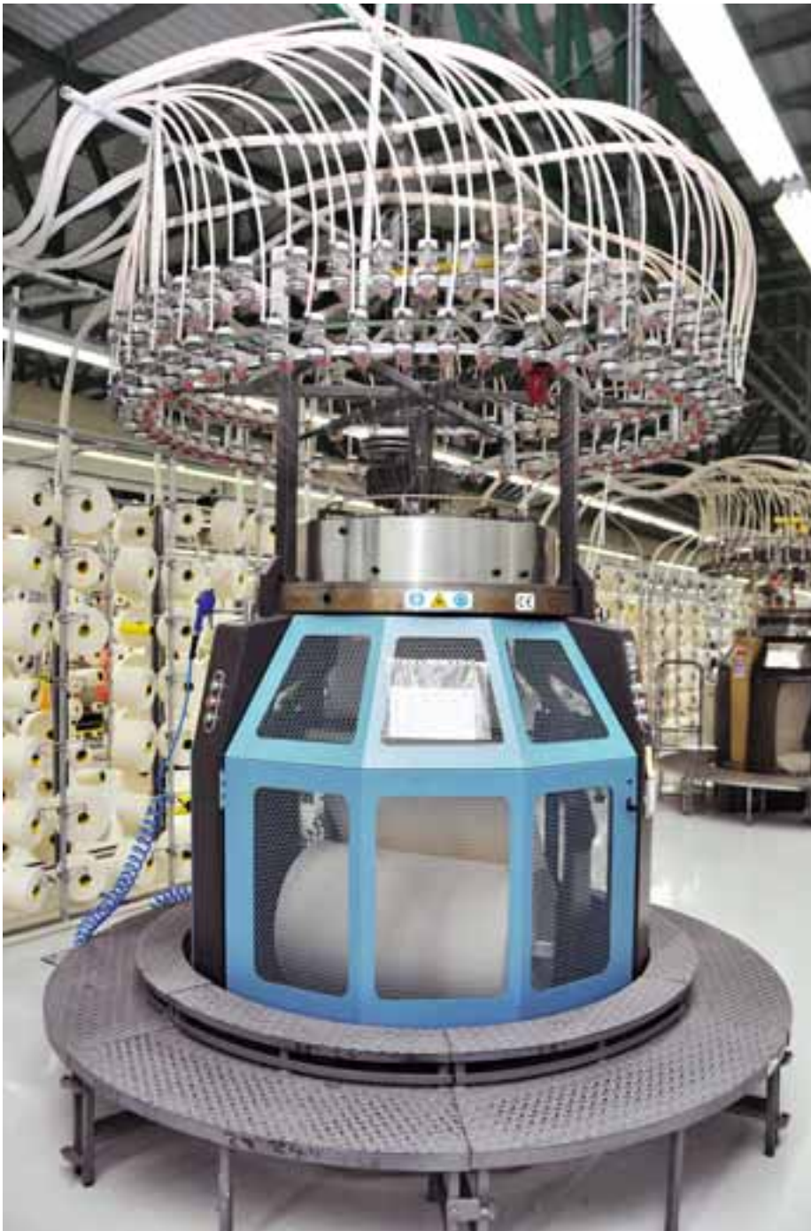
One of the high-speed knitting machines.
