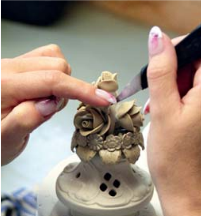
Skilled hands individually shape fine details before the porcelain is fired.
