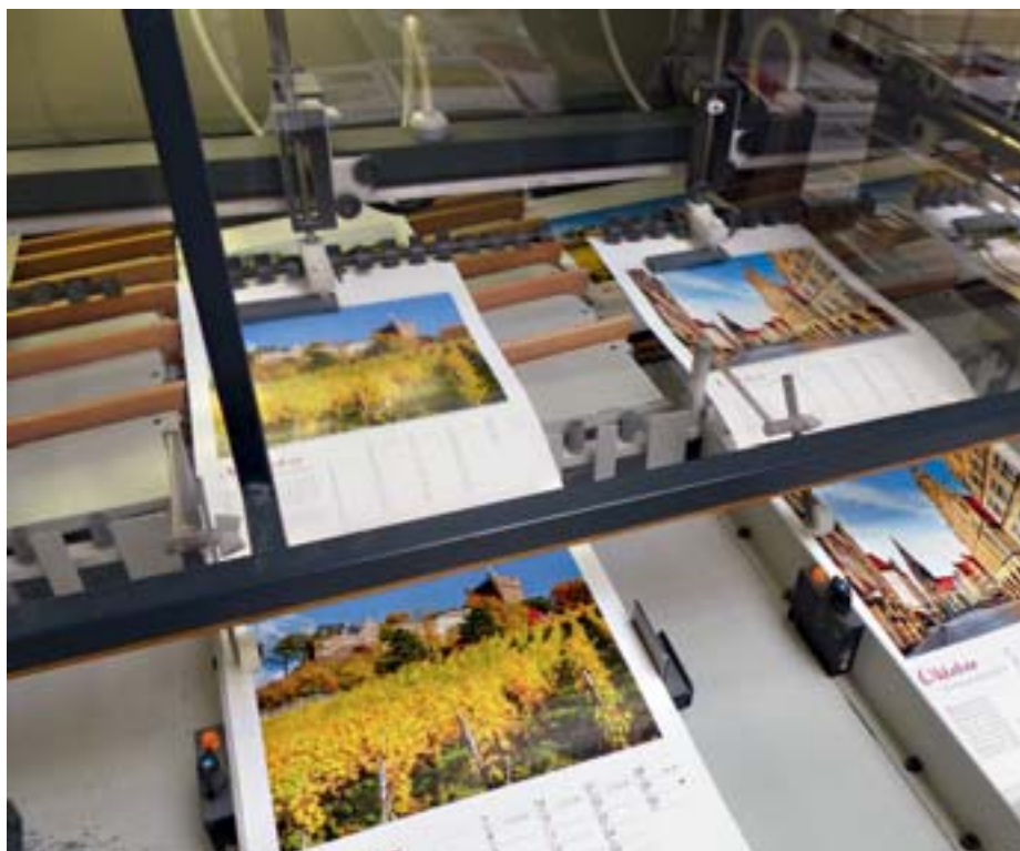
The picture calendar's individual pages are mechanically combined into a complete work.
