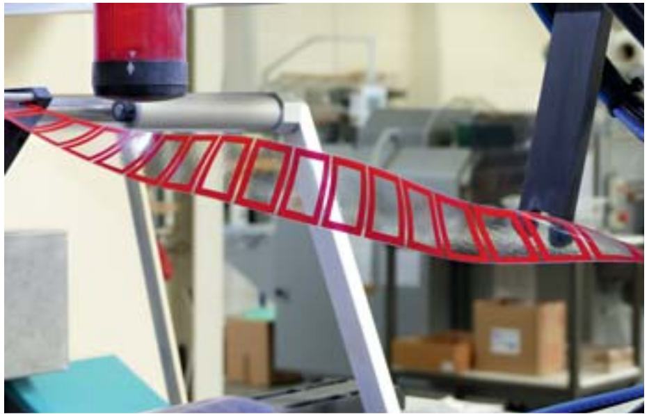
No monthly calendars without date marking. The small, red rectangles for manual date setting must be present.
