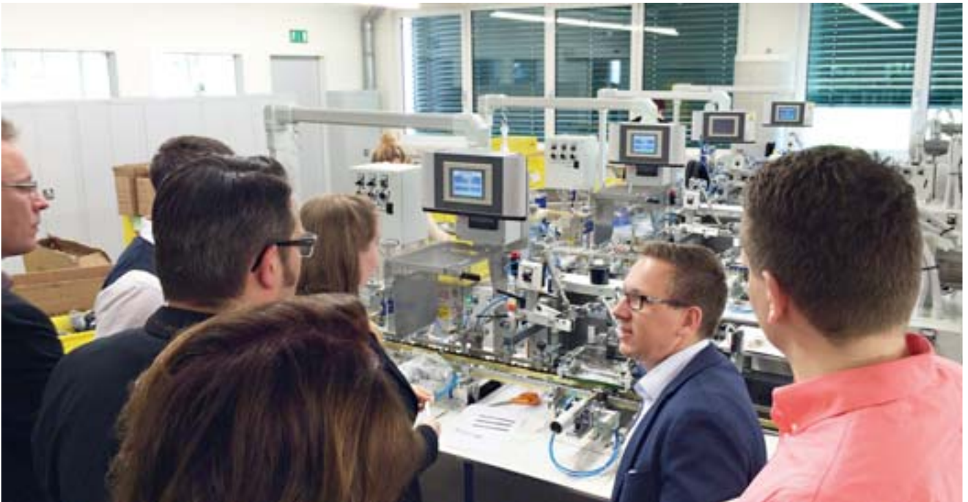
A pad printing press for multicolour prints on writing utensils.
