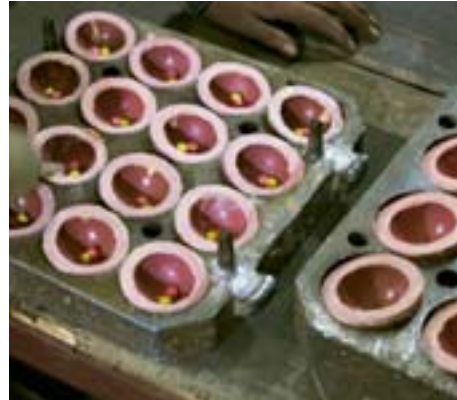
Before the hemispheres are joined together, they are filled with chemical substances which react under hot steam and thus build up a higher pressure in the ball.
