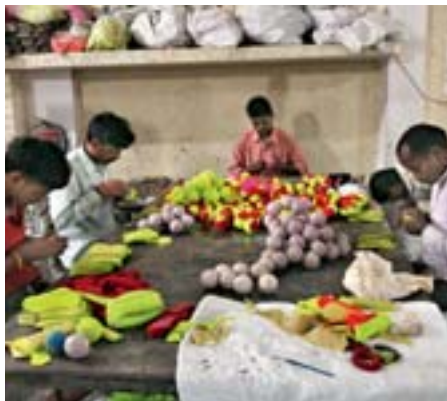
The stamped felt pieces are glued onto the finished natural rubber balls.
