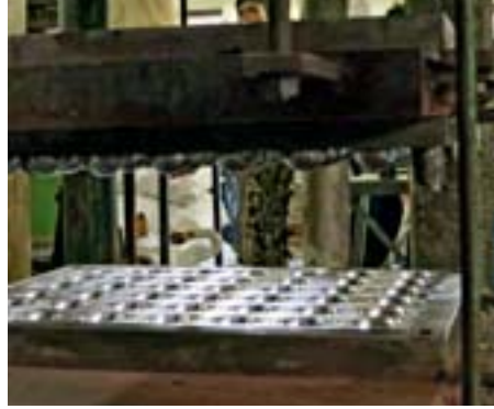
The first step towards a tennis ball: The hemispheres made of rubber are produced in these moulds.
