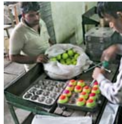
The felt pieces are then bonded with white natural rubber.
