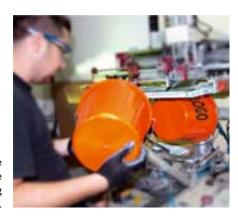
A view of the production: Here buckets are being printed.
