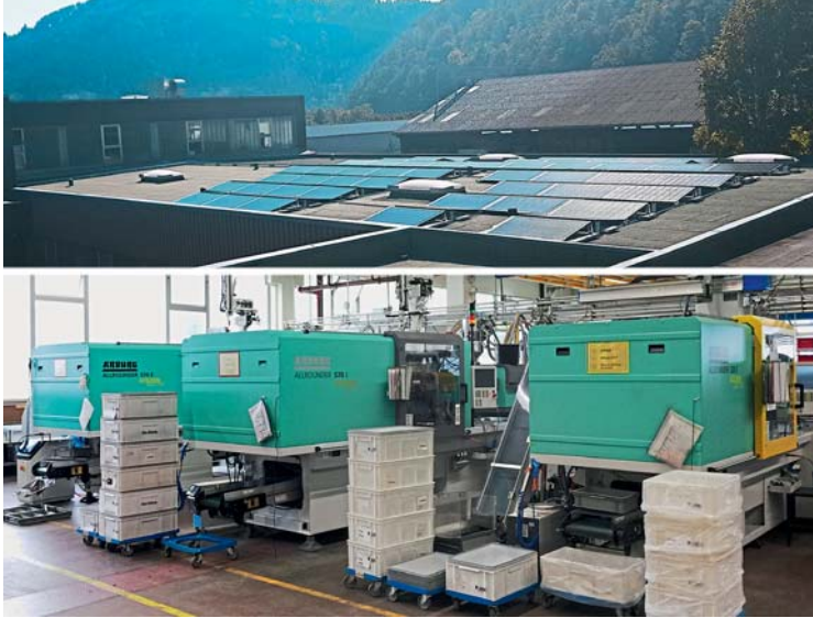
The new photovoltaic system supplies the electrical machinery with “green” electricity.
