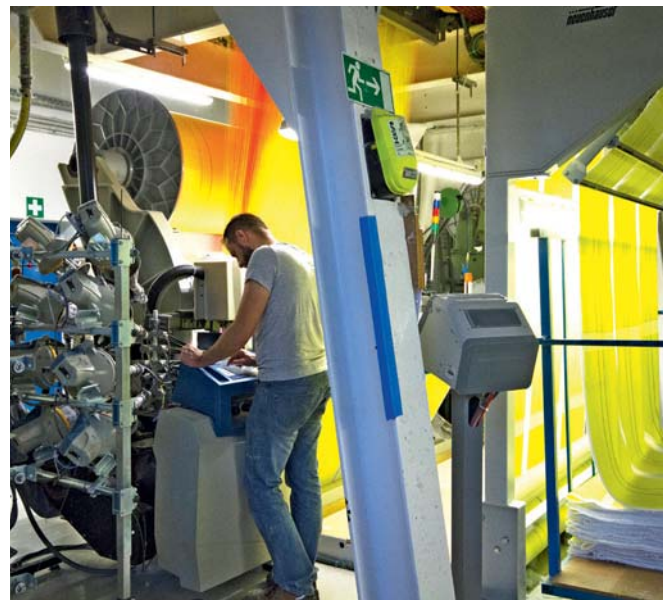
A weaving machine with yellow terry: an expanse of approx. 12,000 towels is produced on a daily basis.
